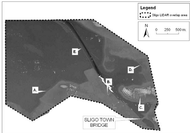
Figure 3. Visualisation of combined OSI, OPW, and INFOMAR LIDAR data for Sligo integrated onto ITM coordinates and Malin datum.
