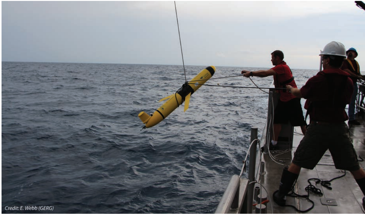
Figure 16.9. Pilot test of an autonomous underwater vehicle for hypoxia studies in the northern Gulf of Mexico by the Texas A&M University Geochemical and Environmental Research Group. Photo by Eddie Webb (Texas A&M University Geochemical and Environmental Research Group).
