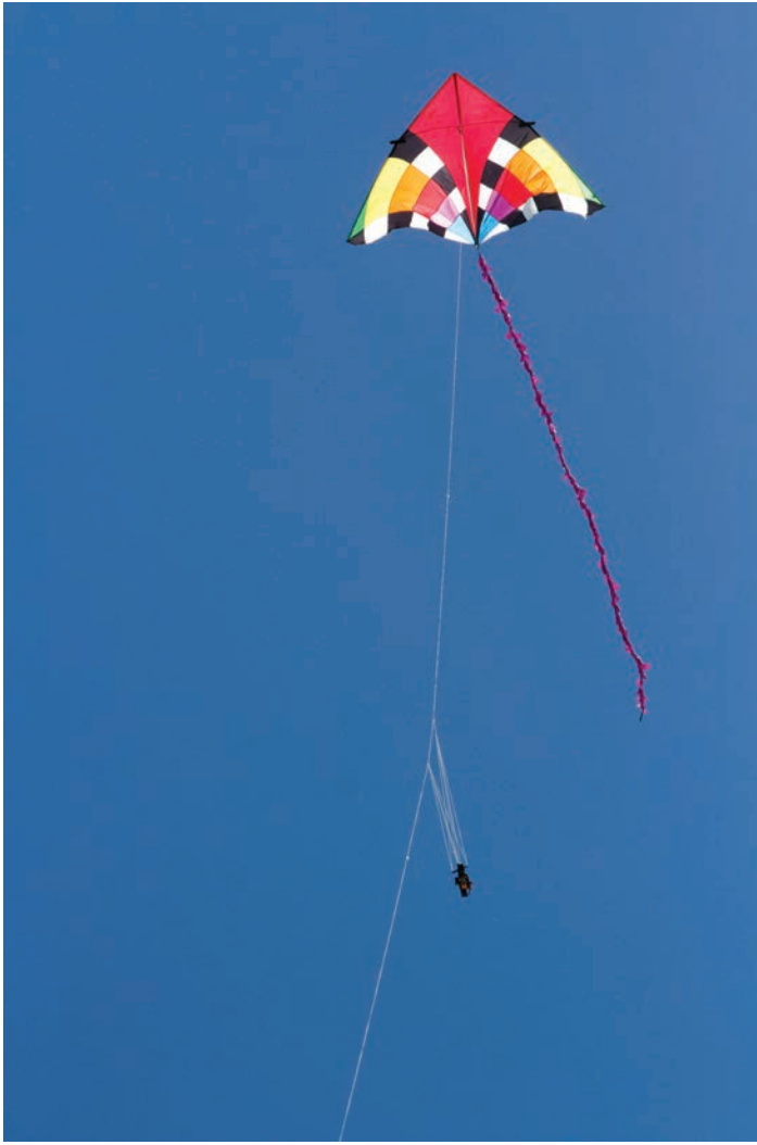
Figure 21.6. The 2014 KAP project used a Pentax Optio WG-2 GPS camera mounted on a 9 ft diameter delta kite with ground control points (GPS) identified using a Trimble GeoXH 6000. High-flight photos were taken at 107 m, and low-flight photos were taken at 54 m with resolution sufficient to capture bird nests on the ground. Photo courtesy of Ian Eland.
