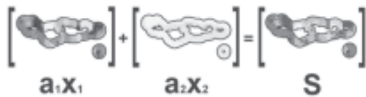
Figure 6.6. Criteria weighting analysis in CI-SSAT. Each criterion data layer ( x_n ) is weighted ( a_n ) according to user values and added to other weighted criterion data layers to produce a base map ( S ).
