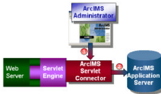
Administrative requests are sent from the Administrator to the ArcIMS Application Server via the ArcIMS Servlet or Java Connector.
