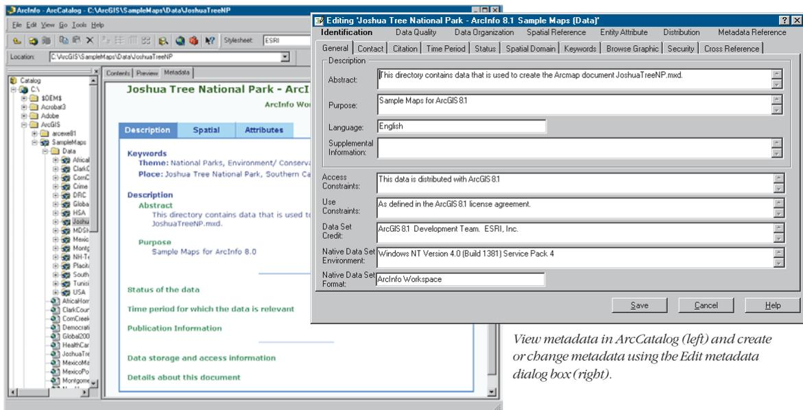
View metadata in ArcCatalog (left) and create or change metadata using the Edit metadata dialog box (right).
