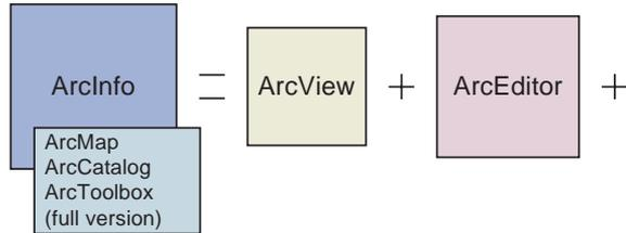
*ArcInfo provides all the capabilities of ArcView and ArcEditor 8.2 as well as additional advanced geoprocessing functionality. The ArcInfo version of ArcToolbox is important for sites that build and create spatial databases.*
