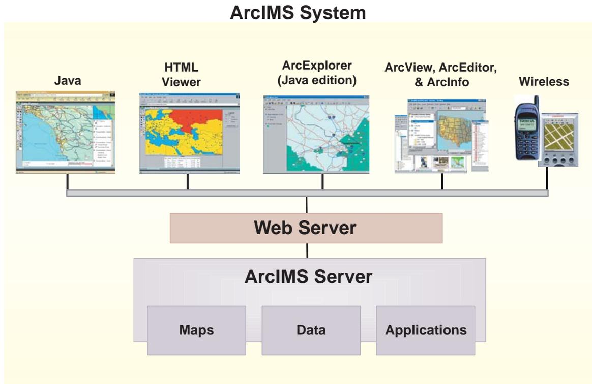
*The ArcIMS system consists of a series of clients (Java Viewer, HTML Viewer, and so on) that access GIS functionality and services provided by an ArcIMS server. Client/Server connections are made over the Internet.*
