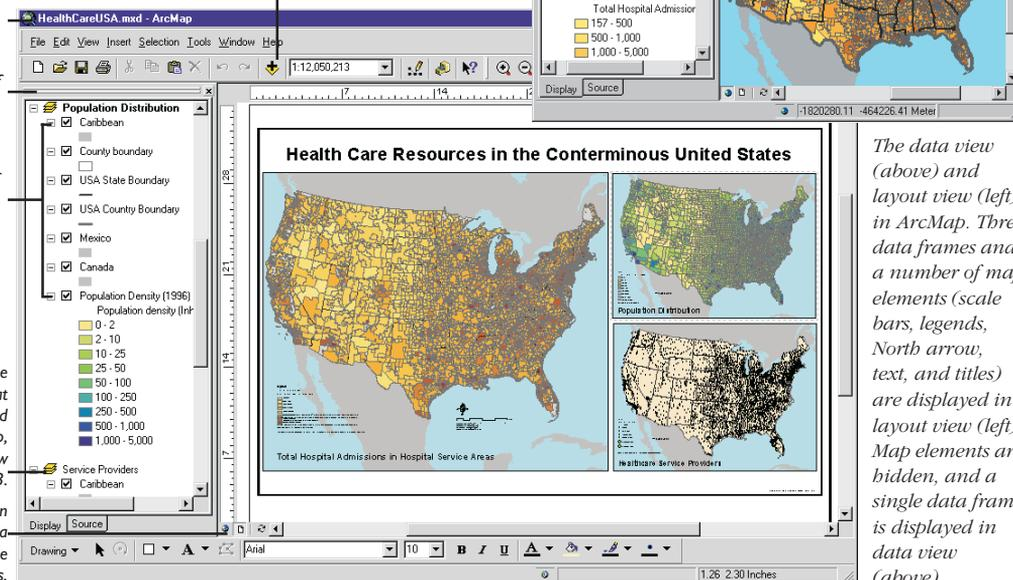
The data view (above) and layout view (left) in ArcMap. Three data frames and a number of map elements (scale bars, legends, North arrow, text, and titles) are displayed in layout view (left). Map elements are hidden, and a single data frame is displayed in data view (above).
