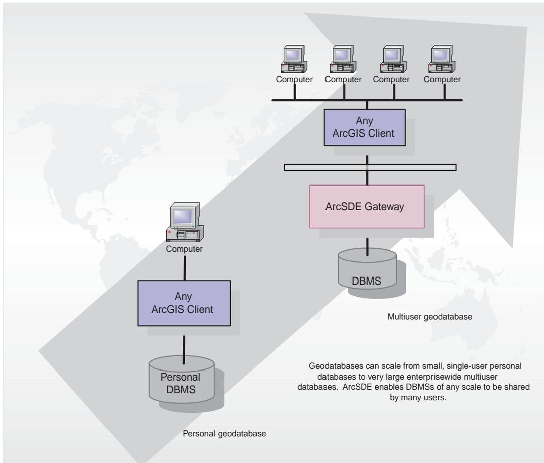
part of the organization's data holdings, and access to this data must be open and easy. The main role of ArcSDE and the geodatabase is to manage the integration between a GIS and a DBMS.
