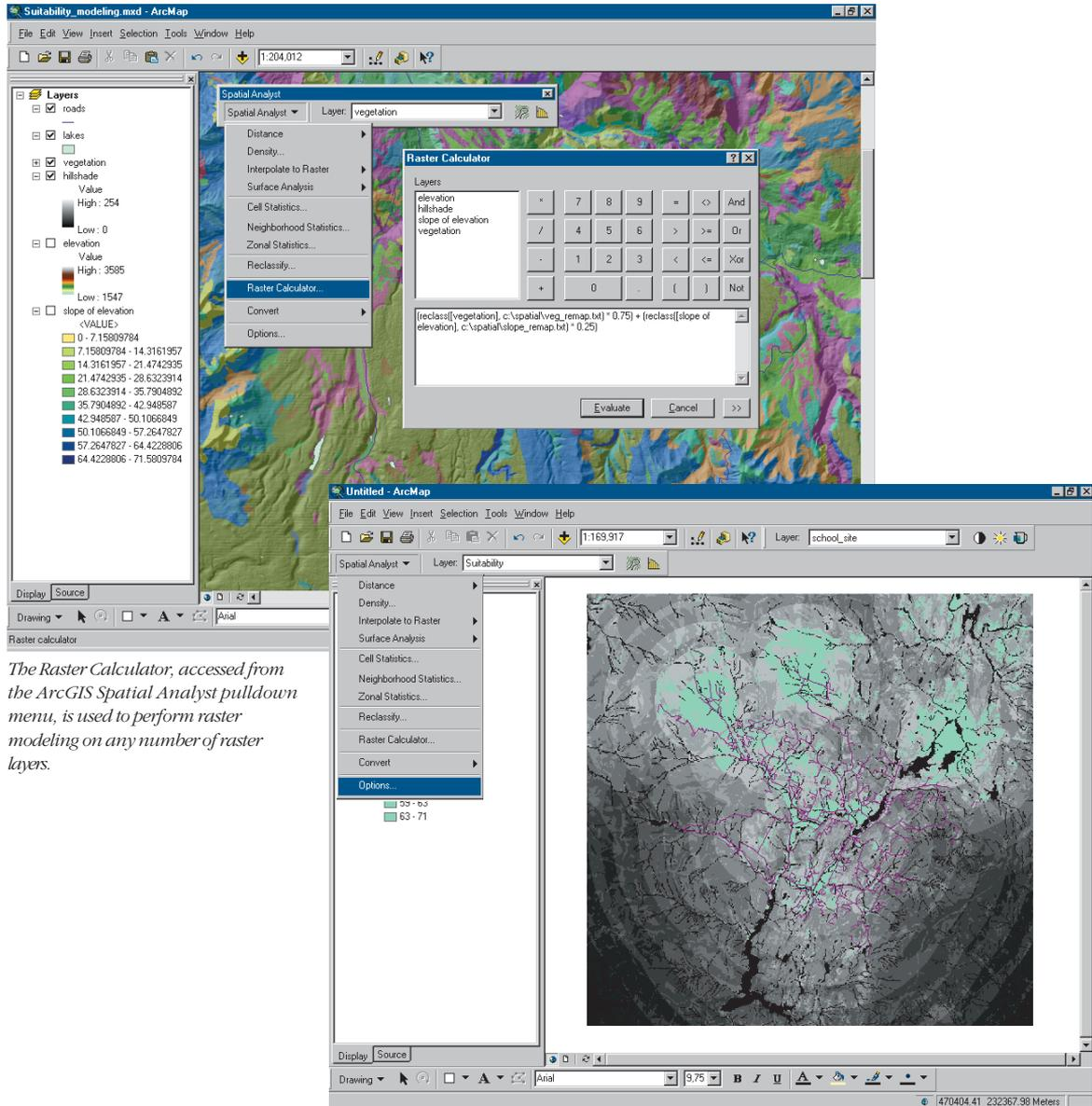
*The Raster Calculator, accessed from the ArcGIS Spatial Analyst pulldown menu, is used to perform raster modeling on any number of raster layers.*
