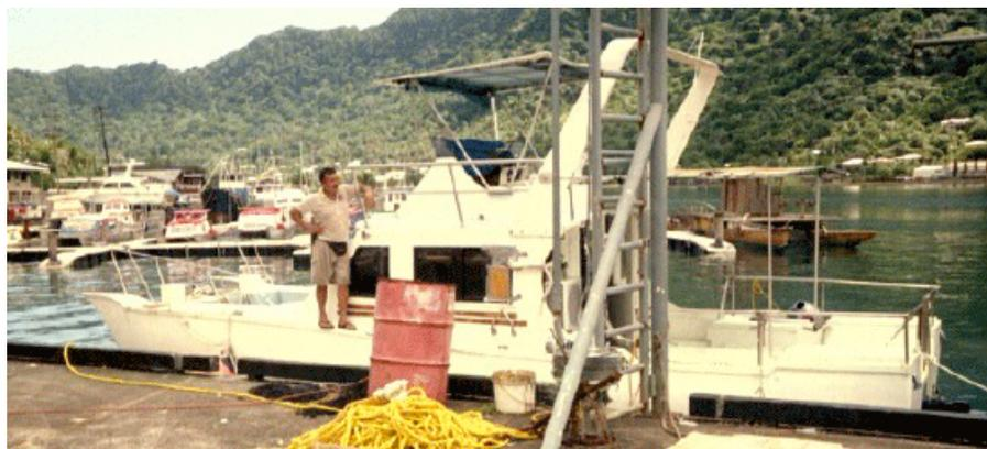
Figure 3.5. 30-foot survey boat of the America Samoa DMWR used for bathymetric surveys.
