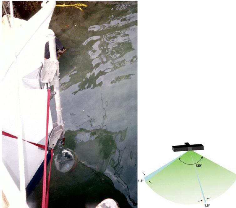
Figure 3.6. The transducer of the Kongsberg Simrad EM-3000 for transmitting and receiving acoustic beams. The transducer was mounted at the end of a metal pole secured to the port side pontoon of the survey boat and then cabled to the data collection and processing unit within the boat's cabin. Graphic to the right illustrates the swath emitted from standard multibeam transducers.
