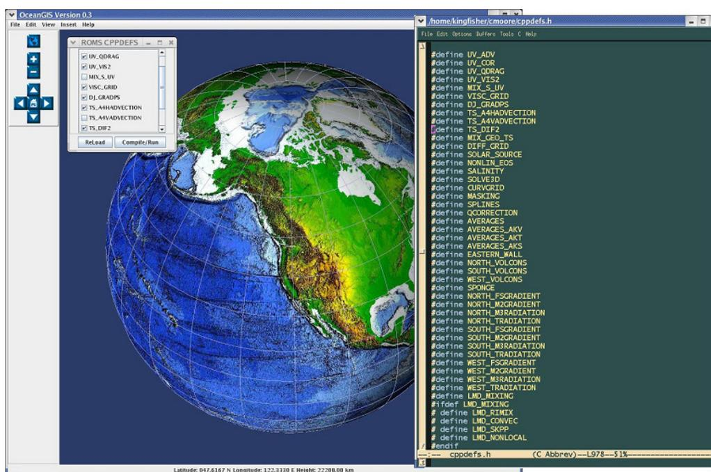
Figure 15 GeoModeler interface to set up preprocessor directives for running the ROMS model.
