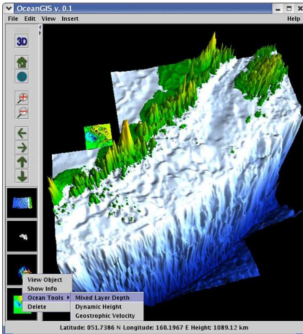
Figure 14 GeoModeler screen shot showing tools for analyzing conductivity-temperature-depth data from the Bering Sea, Alaska. Tools include calculation of mixed layer depth and other oceanographic variables.
