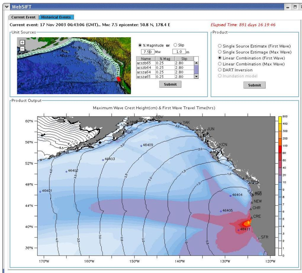
Figure 17 Output from the MOST tsunami propagation model
