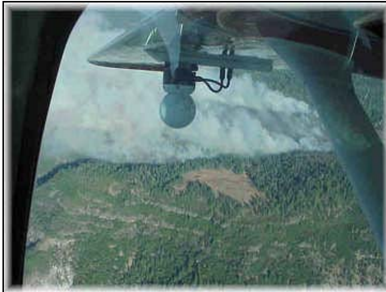
Figure 9—A FLIR system mounted on a fixed-wing aircraft. Source Lassen National Forest.
