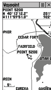
USGS Map Item marked as a Waypoint on a Garmin eTrex Vista
