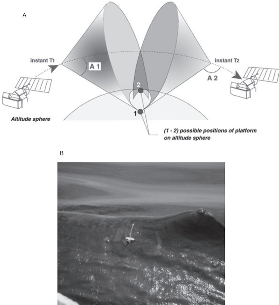
**Figure 2** Top (A): Argos satellites and the solution pair generated by service Argos geolocation, as adapted from Austin et al. (2003) and Liaubet and Malardé (2003). Bottom (B): Photo of Argos satellite tag (~19 cm long) in a sperm whale immediately upon insertion (from Mate et al. 2007)
