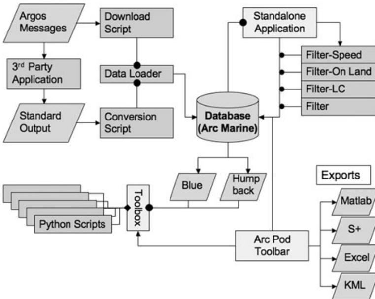
**Figure 10** Conceptual diagram for a future application framework for MMI marine animal tracking data. The framework is centered on the customized Arc Marine database, download and data loader scripts, a standalone application with filter functions, an analytic toolbox with Python geoprocessing scripts, and an integrated ArcGIS extension
