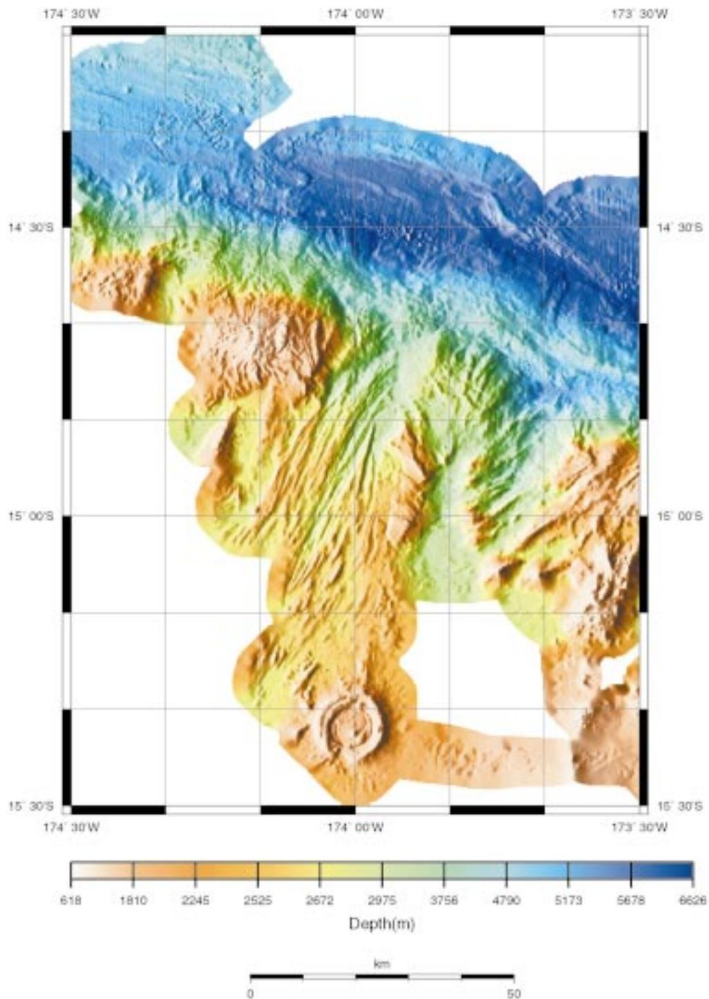
*Figure 7.* Histogram equalized, shaded relief bathymetric map, created from a 200-m Sea Beam 2000 grid (Boomerang 8), of a small ridge-transform boundary to the west of the Tonga Trench. The bathymetry is illuminated at an azimuth of 90° using a shading magnitude of 0.4 to accentuate the spreading fabric of the ridge centered at 174° W, as well as a back-arc caldera at ~15° 25' S, 174° W. Color change interval based on histogram equalization. Map projection is Mercator.
