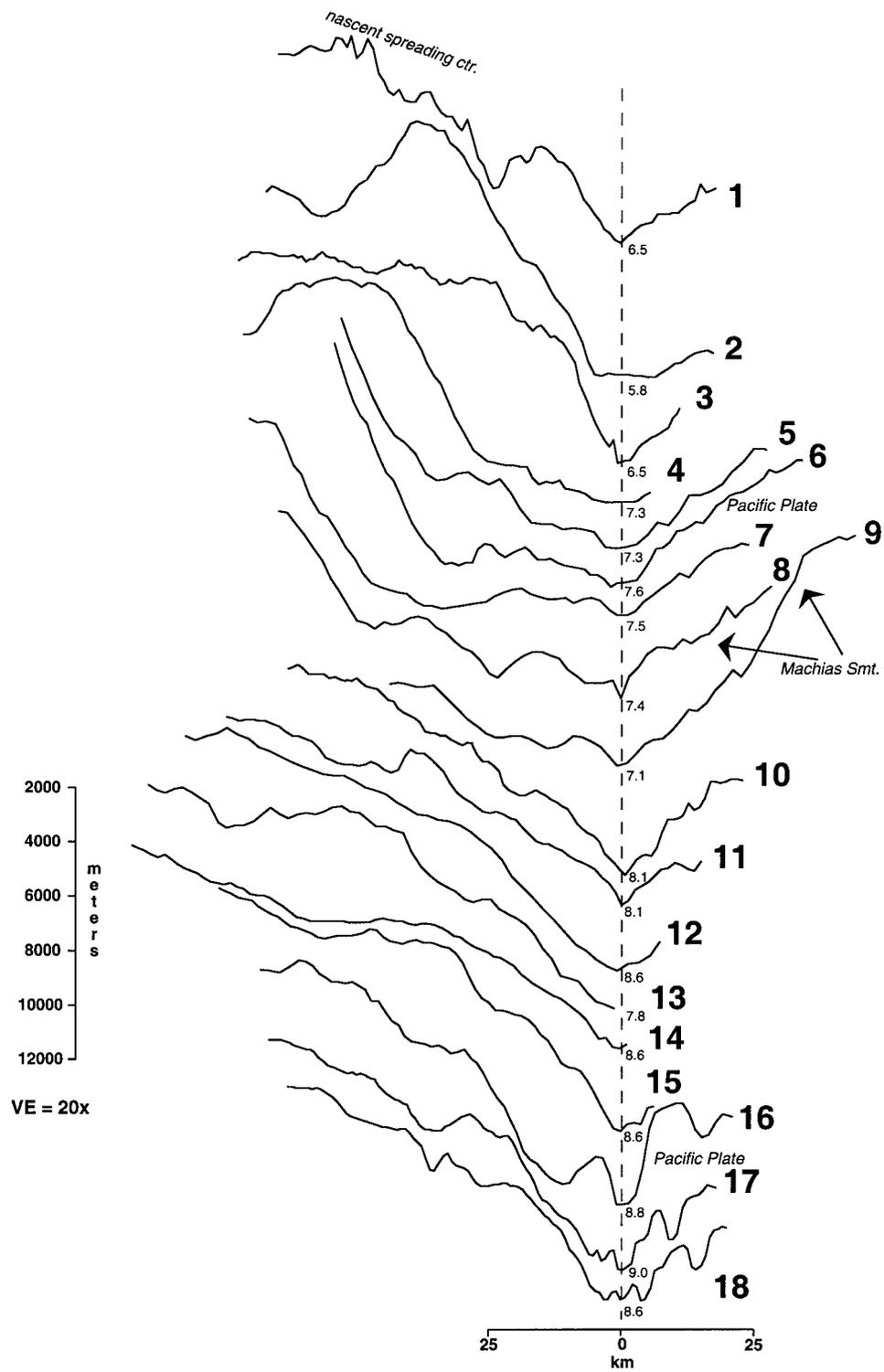
Figure 5. Bathymetric profiles across the northern Tonga Trench and forearc. Profiles are from the center beam of Sea Beam 2000 swaths and have been projected normal to the trench axis. Dashed line shows location of trench axis, and small numbers at bottom of each profile denote maximum depths in kilometers.
