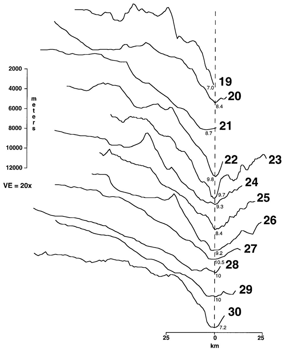
Figure 6. Bathymetric profiles across the central and southern Tonga Trench and forearc. Profiles are from the center beam of Sea Beam 2000 swaths and have been projected normal to the trench axis. Dashed line shows location of trench axis, and small numbers at bottom of each profile denote maximum depths in kilometers.
