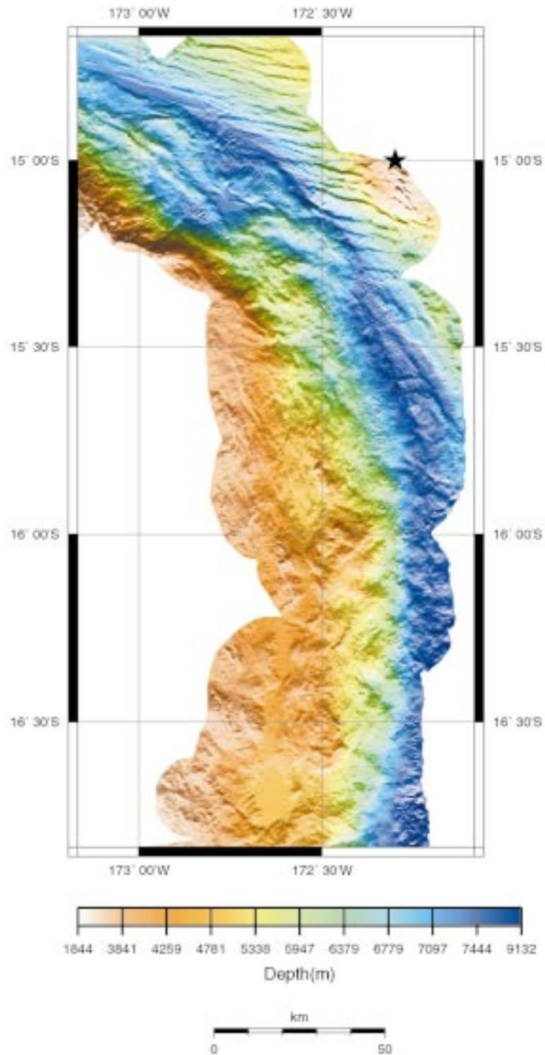
*Figure 8.* Histogram equalized, shaded relief bathymetric map of the northern forearc and westward bend in the Tonga Trench, created from a 200-m Sea Beam 2000 grid (Boomerang 8). Summit of Machias seamount denoted by star. The bathymetry is illuminated at an azimuth of  $0^\circ$  using a shading magnitude of 0.4 to accentuate the abyssal hill fabric at the bend in the trench. Color change interval based on histogram equalization. Map projection is Mercator.
