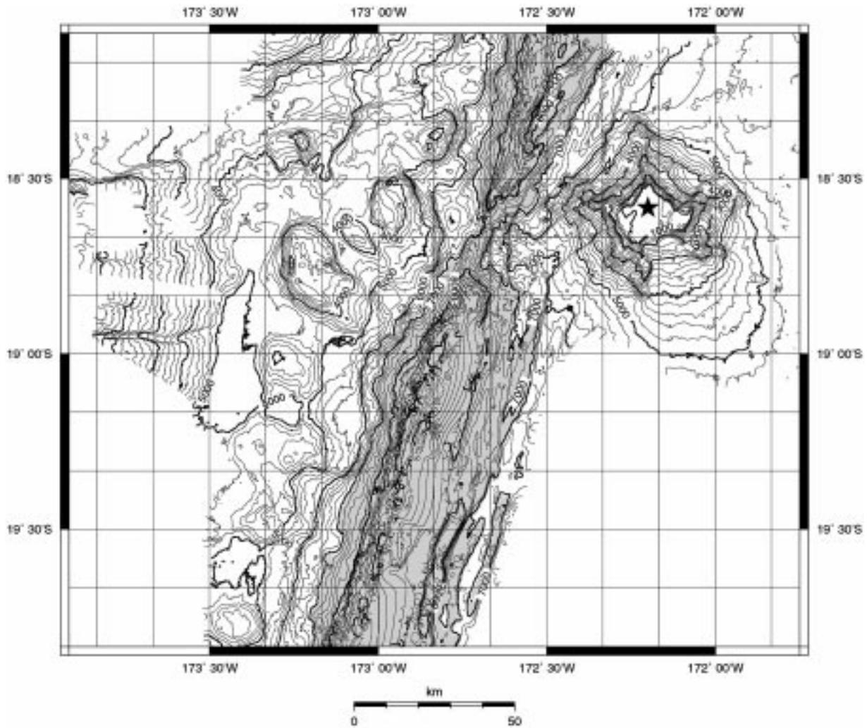
Figure 9. Bathymetric map (200-m contour interval) of the Tonga Trench and forearc, in the vicinity of Capricorn seamount (denoted by star). Shading indicates areas deeper than 7000 m. Note the distinct submarine canyon to the west of the trench at  $\sim 19^\circ$  S. Map was created from a 200-m Sea Beam 2000 grid (Boomerang 8), with portions of the trench axis filled in by Sea Beam data from Marathon 6. Map projection is Mercator.
