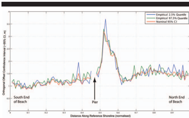
Figure 6. Estimates of horizontal uncertainty using theoretical (scaled standard deviation) and empirical (quantiles of the empirical cumulative density function) methods. Horizontal uncertainty is estimated to be approximately 1.0 m (95%) at the southern end of the shoreline (left), to rise to about 3.3 m (95%) immediately after the pier, and to return to about 1.5 m (95%) at the northern end (right). The small differences among the estimates suggest some small asymmetry of the distribution of offsets about the reference curve and some level of sampling noise due to the small size of the estimation ensemble.
