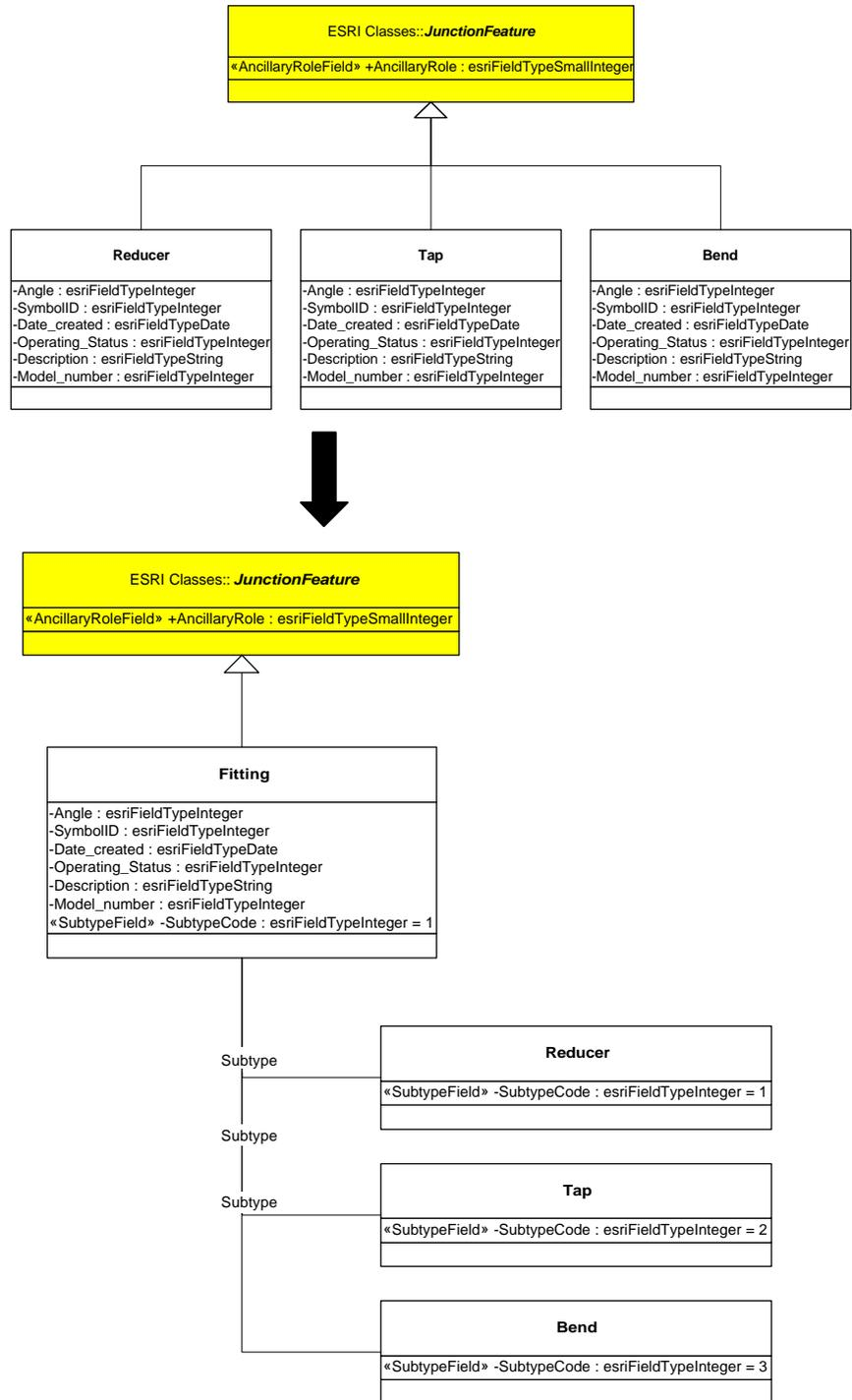
*Reduce the number of classes in your model by lumping them together using subtypes. In this example, three classes, Reducer, Tap, and Bend, were lumped into a single feature class—Fitting—using subtypes.*
