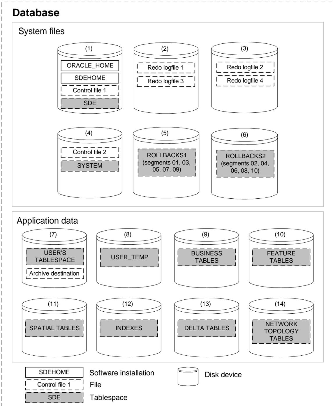
Disk (1) will contain Oracle and ArcSDE executables, the first of two control files, and the SDE tablespace used for our geodatabase's metadata.
